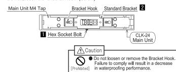
2 Attach the SZ320-KS to the main unit of LED Work Light. Attach an M4 screw to the "Model CLK-24(A)AG mounting hole" and "Main Unit M4 tap". Use a mounting torque of 1.4 N m
