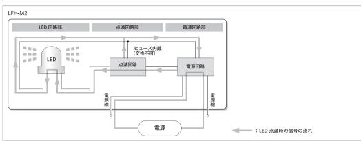
The following illustrates the internal block diagram for the Signal Light. Use it as reference when wiring. (The diagram is only an example.)
